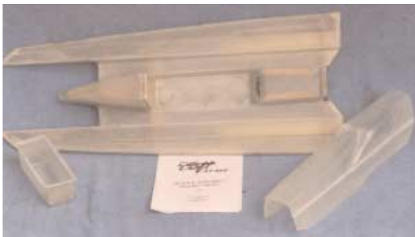
The B&M LeeCraft XT460 comes with a lightweight epoxy glass hull and cowl and a formed radio box.
