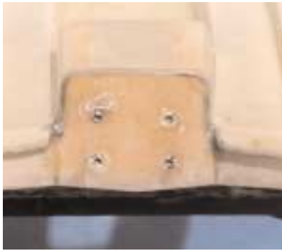
Left: I used threaded brass inserts instead of blind nuts to secure the motor-mounting attachment screws.
