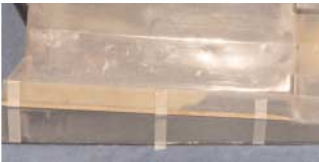
To help cornering performance, I added a strake to the bottom of the left sponson. It is made of a strip of wood that I sanded to shape and glued to the sponson bottom.
